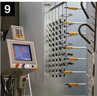
**9** Powder is applied with 18 automated and 2 manual spray guns. Compressed process air is dried to -35°F Dew Point for superior adhesion.
