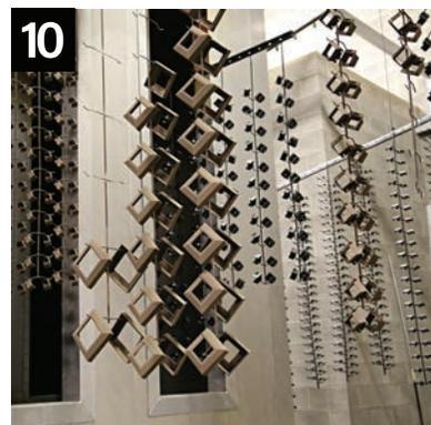
**10** The powder coating is then bonded and adhered to the aluminum substrate in a 400 degree cure stage.
