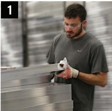
**1** The raw premium-grade aluminum is inspected to be free of blemishes and is not exposed to the outdoor elements.
