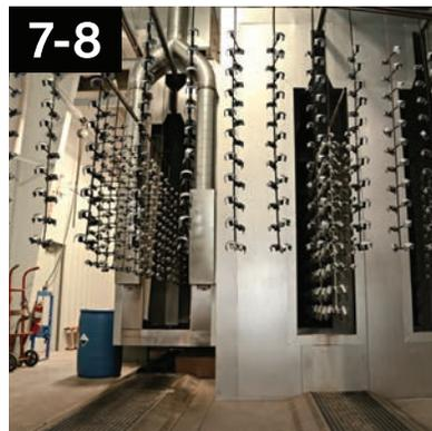
**7-8** A 200 MPH air blast removes water drops from the pre-treated aluminum. A convection oven completes the dry-off process.
