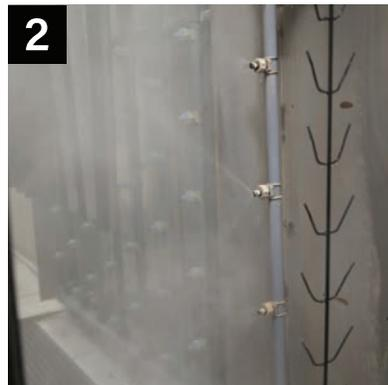
**2** The product enters a heated acidic cleaning stage to remove extrusion debris and fabrication oils.
